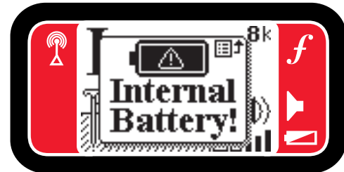
Figure 5 – Internal Battery Alert
