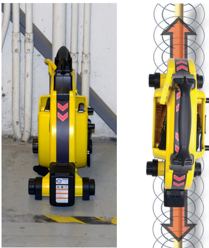
Figure 12 – Orientation arrows aligned with target conductor
