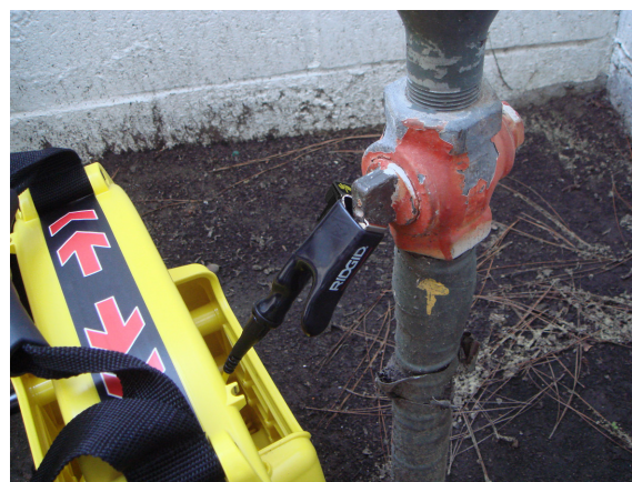
Figure 11 – Connecting the ST-33Q Cable Lead to the Target Conductor
