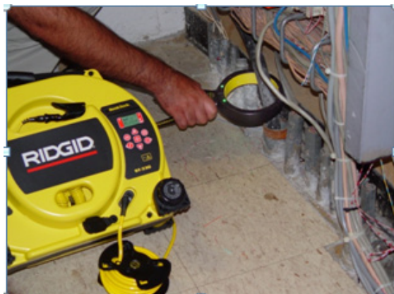
Figure 15 – Inductive Clamp Connected to a Cable
