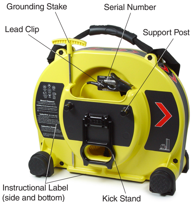
Figure 2 – Back View Transmitter Components
