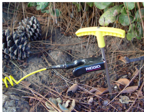
Figure 10 – Attaching the ST-33Q Lead to the Ground Stake
